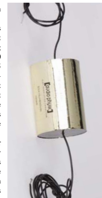
No additional cable: the capacitor contacts are long enough to reach the tweeter.
